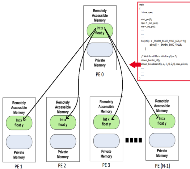
Fig. 4: Diagram of a simple broadcast operation.
